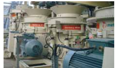
Stationary : One HP500, one HP300, two HP200 crushing "Amphibolite".
