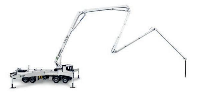
Thanks to the easy to operate RZ system and large opening angles of the boom stages 4 (235°) and 5 (230°), the S 51 SX is extremely flexible and safe during operation. Further benefits are the low unfolding height of just 9.80 m and large slewing range of 2 x 365°. To increase safety when pumping and to minimise the danger of blockages, only standard elbows with a large radius and camber of 275 mm are used with the boom pipes of the S 51 SX.
